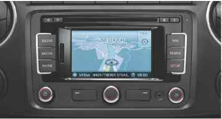
RNS 315 5" colour touch-screen. 6GB flash memory. FM/AM radio with RDS. Single CD player. AUX-IN and SD card slot. Western European data. 6 speakers.
